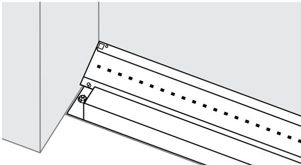
**STEP 3:** The next fixture in the row can be set in place and will interlock with the previous fixture by use of tabs.
