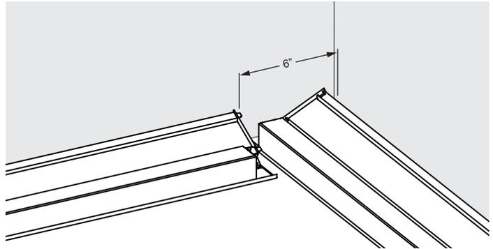
**STEP 7:** The CX lens (packed separately) is provided in 96" sections. Simply lay the lens in place within the channel as shown. The last lens placed should be cut to the proper length utilizing a standard miter saw or miter box to provide an accurate fit.
