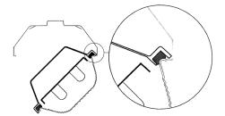
STEP 3: Push up on the enclosure and then press in on the mounting bracket until the mounting bracket clicks into place.
