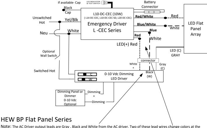
Note: The AC Driver output leads are Gray, Black and White from the AC driver. Two of these lead wires change colors at the LED connector. The changed colors are Red (+), White (W) and Gray. The Red and White wires must be cut and wired as shown to the L Series LED EM Driver. Do not cut the Gray wire.
