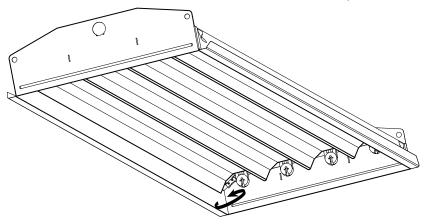
STEP 4: Confirm correct lamp orientation on sockets based on fixture "N", "L" marking.
