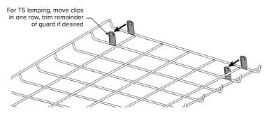
STEP 2: Attach the clips to the end plates of the fixture using #8 screws supplied.
