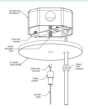
STEP 1: Mount the cross bar bracket to the junction box.
