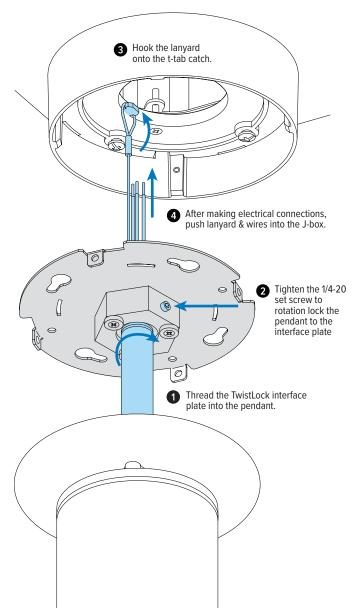
B. Make power input and dimming control electrical connections in accordance with NEC and local codes. Low-voltage lead terminations for cylinders with remote driver box.
