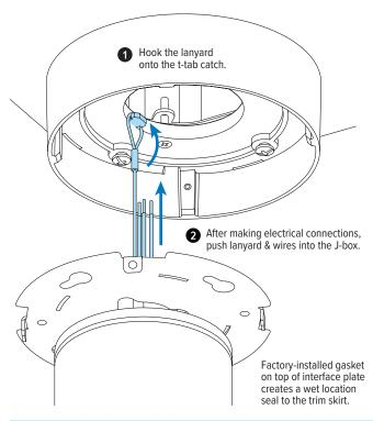
B. Make power input and dimming control electrical connections in accordance with NEC and local codes. Low-voltage lead terminations for cylinders with remote driver box.
