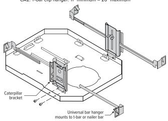
FIG 1.2 BA1 Butterfly bracket only | BA2 Heavy-duty universal bar hanger, shown
