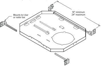
FIG 1.3 Adjustable caterpillar pan bracket
