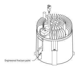
STEP 9: Connect downlight insert to power.
