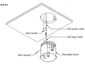
STEP 10: Install downlight insert to ceiling.
