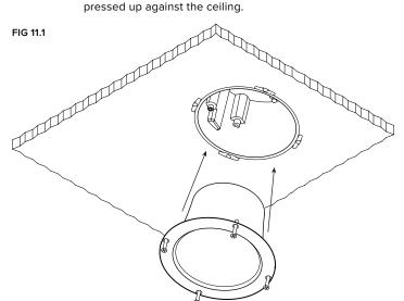
**B.** Drive trim screws until they engage with threaded insert in retainer ring.
