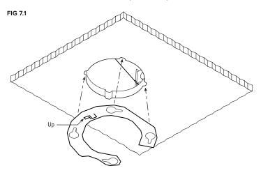
**B.** Lay retainer ring onto pan, with large holes passing over the (4) wing nuts.
