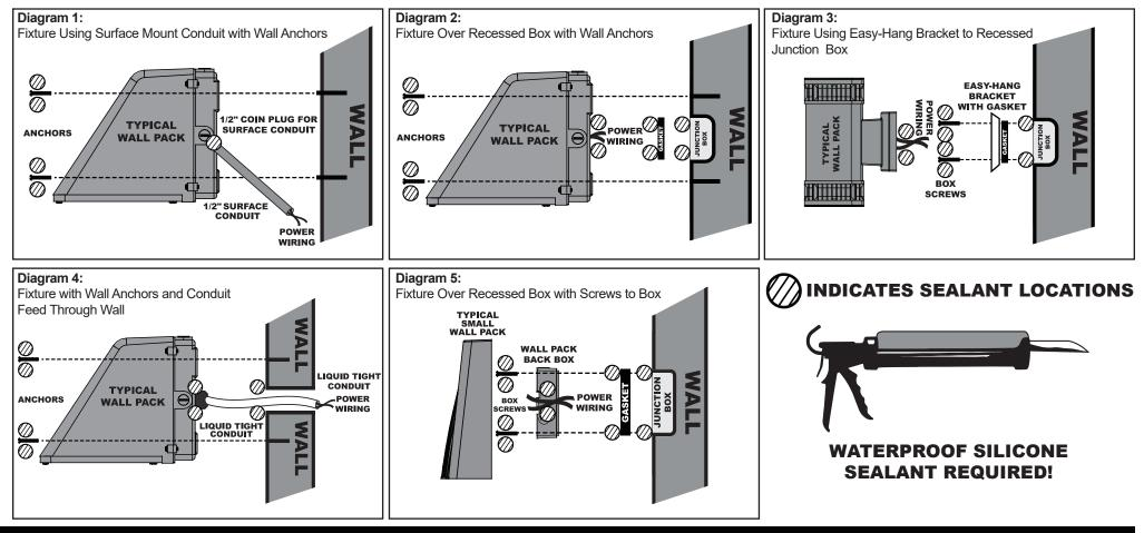
FAILURE TO COMPLETELY SEAL FIXTURE WILL VOID PRODUCT WARRANTY
