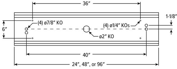
Midsection punching for 4' and 8' units only. 8' unit consists of duplicate 4' unit punching.
