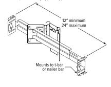
CA2 Adjustable caterpillar pan bracket, t-bar hanger included (N Mounting Type only)
