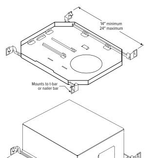
BA1 Adjustable butterfly pan bracket, bar hanger not included (N Mounting Type only)
