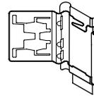
**BA2** Adjustable butterfly pan bracket, heavy-duty universal bar hanger included (N Mounting Type only)
