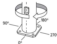
The Radial Index references how parts are oriented around the shaft. A degree measurement is used from a base point. The standard base point of reference is the access door. Degrees are measured in a clockwise motion as viewed from the top of the shaft.
