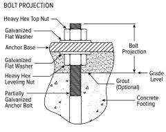
ANCHOR BASE ø11-1/2" Bolt Circle 12-1/16" ø7-1/2″ 1-1/4" x 1-3/4" Bolt Slots
