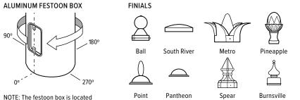
NOTE: The festoon box is located above the access door at 0°.
