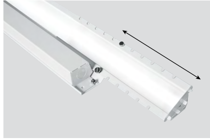
Adjustable to the inch. Fixtures utilizing extensions (EXTL/EXTR) are intended for end of row use only. If connection is required, it must be made on site utilizing flexible conduit.
