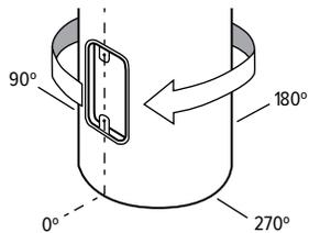
NOTE: The festoon box is located above the access door at 0°.
