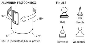
NOTE: The festoon box is located above the access door at 0°.
