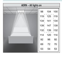
Footcandle calculations based on standard reflectance of 80/50/20 and a light loss factor of .85. Fixture centered over bed at 9' ceiling height, positioned 4' on center from wall. Values are for bed surface.
