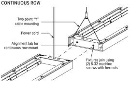
For continuous row mount, suspend fixture using aircraft cable at every fixture intersection and at both ends. Make the electrical connections using the plug-in wiring harness (provided). Install end plates on each end of the continuous row. Depending on installation method, cable mounting may require additional counter-weights due to side-mounted driver.
