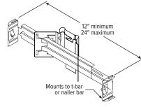
CA2 Adjustable caterpillar pan bracket, t-bar hanger included (N Mounting Type only)
