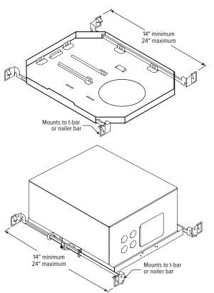
BA1 Adjustable butterfly pan bracket, bar hanger not included (N Mounting Type only)
